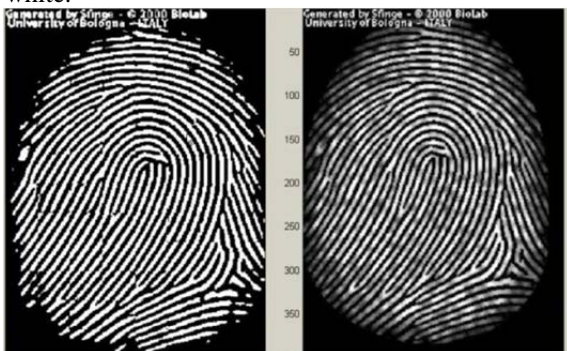
Fig.9 the Fingerprint image after adaptive binarization Binarized image (left), Enhanced gray image (right).
