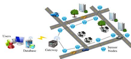
figure 1. the architecture of the proposed automatic micro-scaled air quality monitoring system
