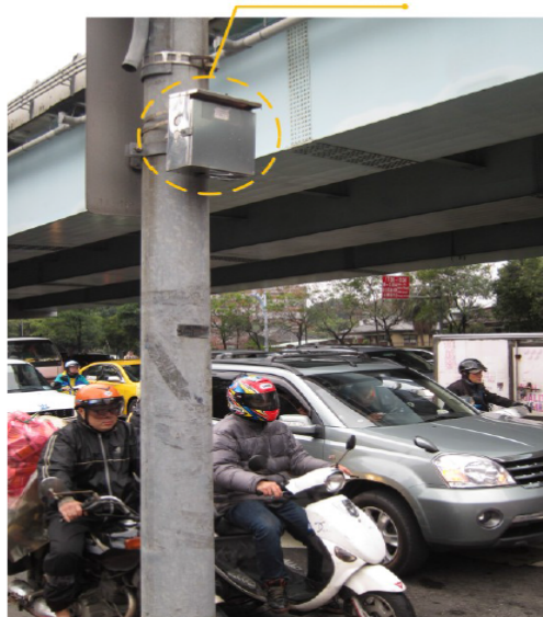
Figure 11. Deployment of the air quality monitoring system. A sensor node was attached to the traffic signal pole
