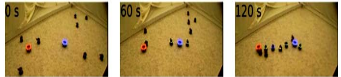
Fig 11: A picture of S-bots forming a chain from the nest to the prey
