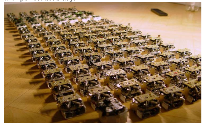
Fig 5: A swarm of robots together in a group to maintain a communication link among themselves
