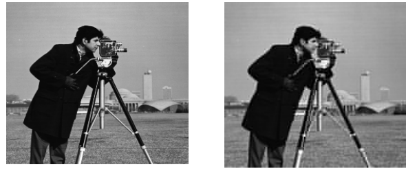
Figure 5: a) Original Image Of Cameraman b) Reconstructed Image after applying 8 x 8 block subset using DCT
